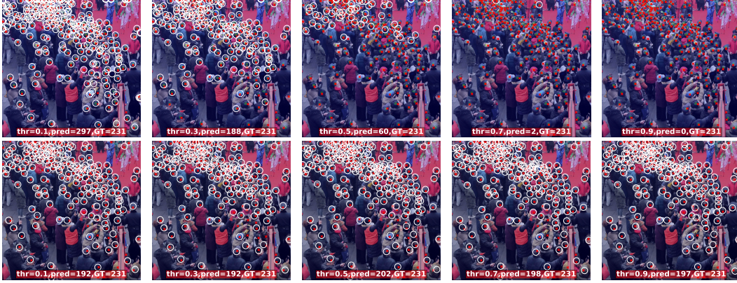
Figure 2: The effectiveness of using diffusion models for localization. The top row is the baseline prediction and the bottom row is our method. The threshold is increasing from left to right. The baseline predictions change dramatically while our prediction is more robust to the threshold. Note that the red crosses indicate the ground-truth and the white circles are predictions.
