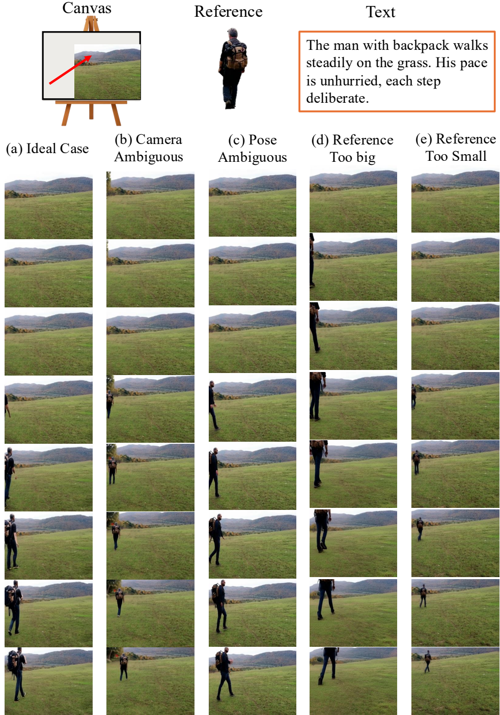
Figure 11: Limitations. Given the same input and conditions, our model may produce different outputs under different random seeds. We consider (a) to be an ideal case and illustrate several limitations: camera motion ambiguity in (b), ID reference pose ambiguity in (c), overly large reference objects in (d), and overly small reference objects in (e).
