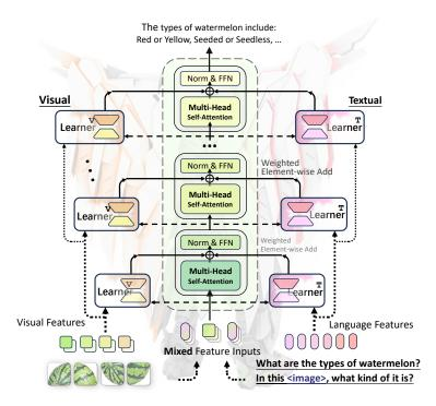
Figure 3: **The WINGS - model architecture.** We introduce extra modules parallel to the main attention, serving as boosted learners to compensate for the attention shift. We train the visual learners on one side, alleviating some shifted attention. Then, we collaboratively learn visual and textual learners based on routing shifted attention weights. They are like light feathers woven "wings".
