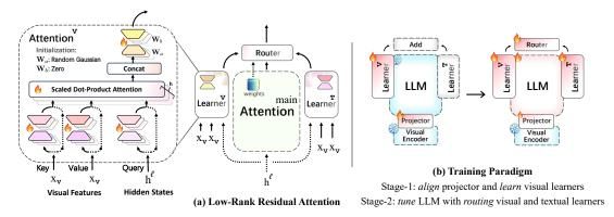
Figure 4: **Illustrations of the detailed WINGS structure, and training strategies.** WINGS is constructed by the Low-Rank Residual Attention (LoRRA) module where the previous hidden state acts as the query and the visual/textual features serve as the key and value. Training starts with visual learners and projectors, followed by the dynamic attention-based routing.
