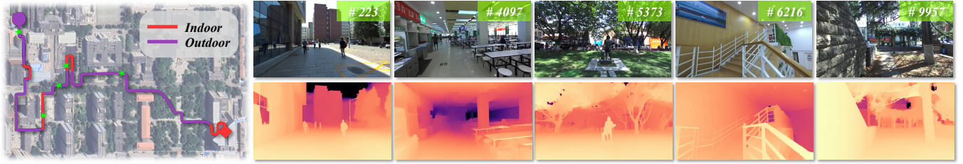
Figure 5: Top view of the scene where we collected the BUPT Depth dataset. Red lines indicate indoor scenes and purple lines indicate outdoor scenes. We give five images and their ground truth depth calculated by CREStereo [26] as examples.
