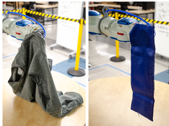
Fig. 1: Holding various flexible objects during manipulation using a 90 degree orientation for the gripping device, with a supply pressure of 300 kPa for the vest and 100 kPa for a piece of textile.
