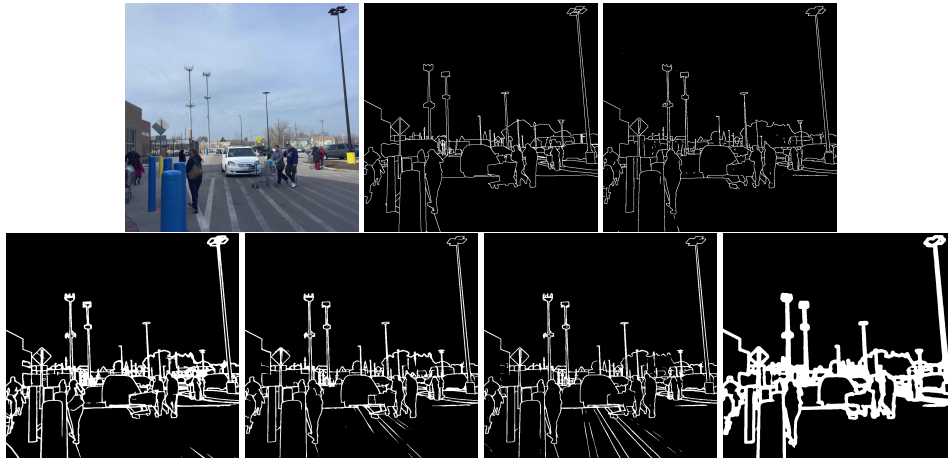
Figure 3: Qualitative comparison between methods on a Mapillary Vistas image from the test set. From left to right on the first row: the original image, the ground truth and the prediction using VT. On the second row: the prediction using WCL, DCL, DL, and DT.
