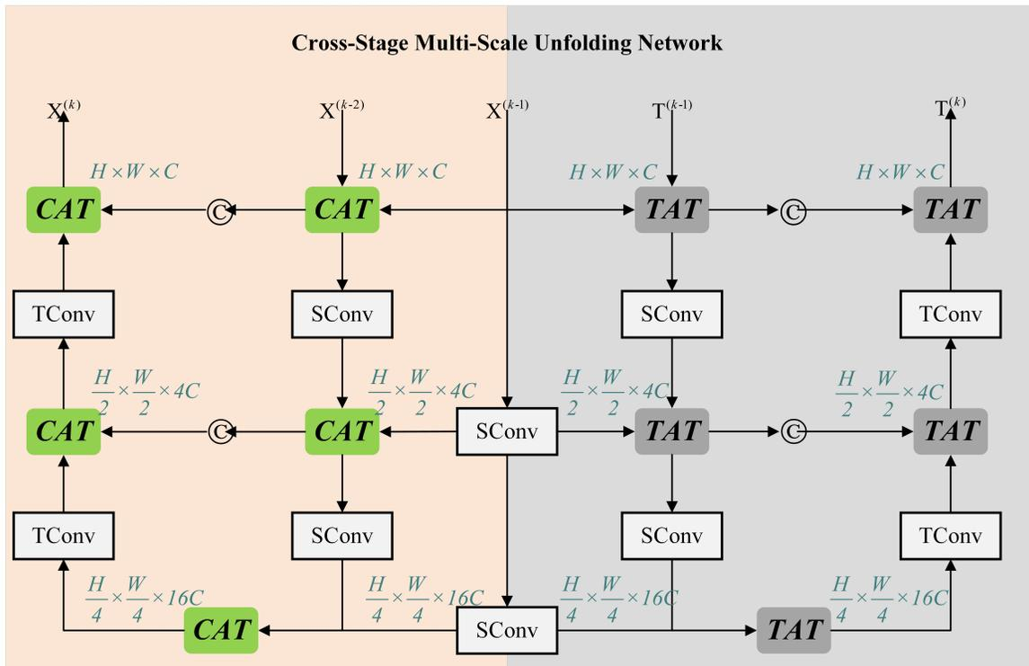
Figure 2: Architecture of our cross-stage multi-scale unfolding network  $\mathbf{D}$ , which consists of a three-scale  $\mathbf{W}$ -shaped backbone, in which the last two scales are equipped with skip connections.  $\mathbf{D}$  is built by multiple CATs and TATs. The strided convolution(SConv( $\cdot$ )) and the transposed convolution(TConv( $\cdot$ )) are adopted as the downscaling and upscaling operators.
