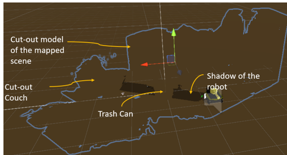
Figure 4: A transparent model of our working scene with robot shadows to be superimposed onto the real-world
