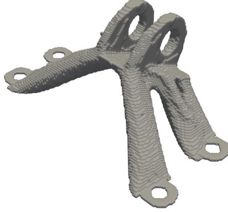
Figure 10: A solution to the jet engine bracket problem found by the FeniTop (Jia et al., 2024) topology optimization software. The quantitative metrics are reported in Table 7.
