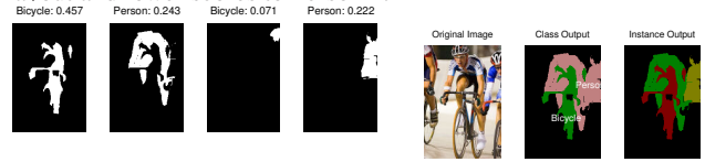
Figure 9. Final masks and final output of the algorithm. Bike 2 is filtered out because of very low score. Superpixels are chosen according to the procedure in Sec. 4. It is interesting to see that the first person has his right leg correctly cut through by the bicycle, a solution that was not available in any of the initial object segmentation proposals.
