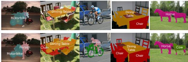
Figure 10. Example of semantic segmentations. The first row shows results using the post-processing algorithm of (Li et al., 2010), the second row shows results of the proposed CSI algorithm. Note CSI performs significantly better in complex scenes with multiple interacting objects.
