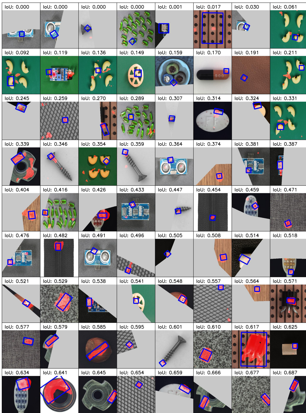
Figure 5: Demonstration of ordered IoU values between prediction (red) and bounding box label (blue). Random images from various MVTEc and VisA classes, with predictions created using the PatchCore algorithm (Roth et al., 2022). We recommend an IoU limit of 0.3, as we propose that from this point onwards (the third row), the prediction and bounding box have satisfactory overlap. Note the gray area means ignored pixels, due to there being other closer anomalies in the given image (see above for explanation).
