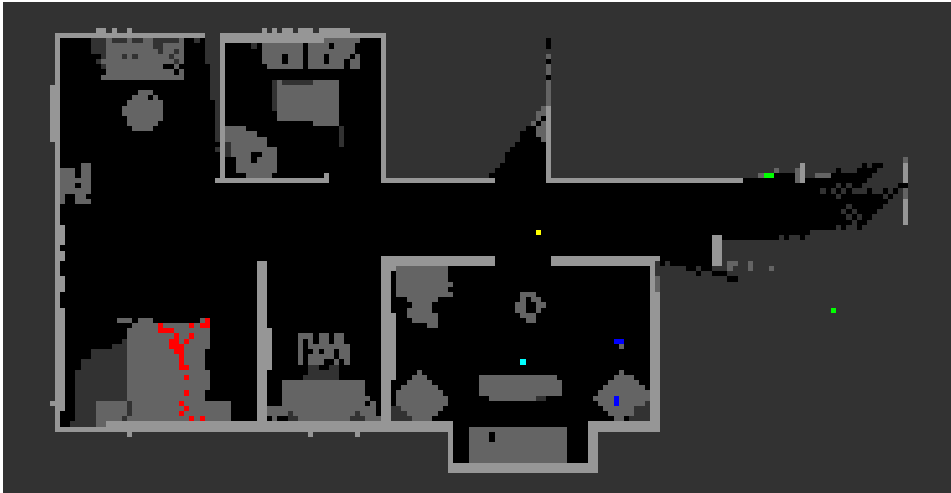
Figure 6: A visualization of the semantic map stored in the Semantic Memory and updated with new observations at every time in the TDW-MAT environment. The destination is shown in red, target objects are in blue, containers are in green, the agent is denoted with cyan, and the other agent’s position in memory is denoted in yellow.
