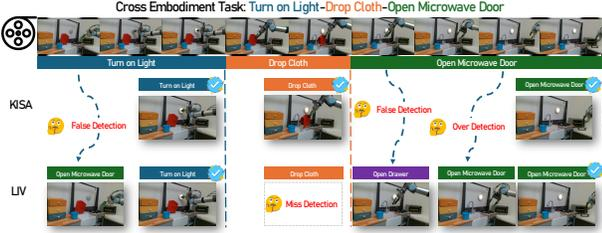
Figure 6. Cross Embodiment Generalization (L3). The illustrating example of LIV and KISA for zero-shot generalization from simulators on long-horizon real robotics demonstration datasets.
