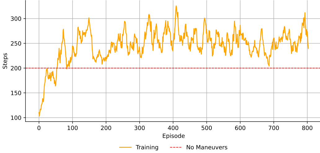
Figure 16: Steps per episode, averaged by a sliding window of 10 episodes. If no maneuvers are executed, the satellite exits the allowed tolerance range by step 200.
