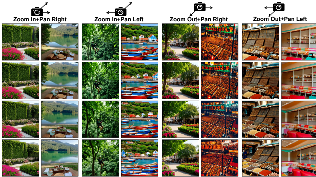
Figure 4: Camera motion combination results: The extracted camera motions can be combined to form new camera motions. The newly constructed camera motions in this figure contain both zoom and pan camera motions at the same time.
