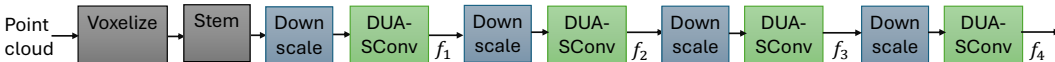
Figure 5: DUA-SConv Based Backbone. Detection head uses only final-stage features ( f_4 ), while segmentation head uses multi-scale features ( f_1-f_4 ).
