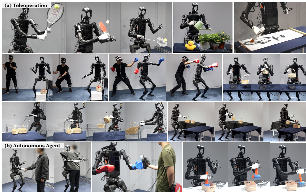
Figure 1: (a) OmniH2O enables teleoperating a full-size humanoid robot (Unitree H1) to complete tasks that require both high-precision manipulation and locomotion. (b) OmniH2O also enables full autonomy through visual input, controlled by GPT-4o or a policy learned from teleoperated demonstrations. Videos: see our website: https://omni.human2humanoid.com
