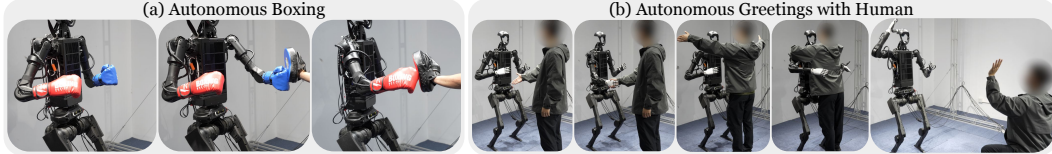
Figure 6: OmniH2O sends egocentric RGB views to GPT-4o and executes the selected motion primitives.
