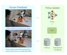
Figure 2: A human operator supervises policy training and provides intervention with a 3D mouse.
