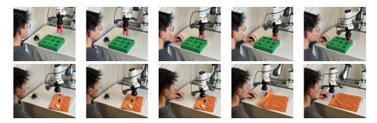
Figure 5: Sequential steps of robot manipulation for the peg insertion and cloth unfolding tasks on a real robot.
