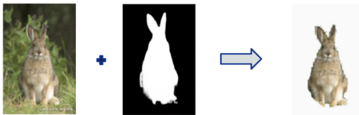
Figure 4. Illustration of how for each image in the ImageNet training set (left) we use our unsupervised version of DeepUSPS to obtain the saliency mask (middle) which we then apply on top of the image to obtain the image with the background removed (right).
