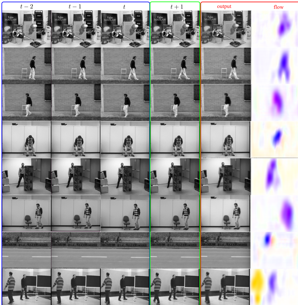
Figure 7: Qualitative results on real videos. The first three columns show the last frames (out of 12 in total) fed into the network (from t - 2 to t ), the t + 1 column shows the ground truth next frame, and the last two columns show the predicted next frame and the predicted optical flow.
