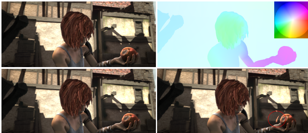
Figure 3: Warping performed by the GG and S modules, given a video frame and the ground truth optical flow map. First line: input frame and ground truth optical flow map displayed using the colour code shown in the top-right corner of the image; the colour encodes the direction of movement and the colour intensity reflects the magnitude; darker shades correspond to higher magnitudes (Baker et al., 2011). Second line: ground truth next frame and sampled next frame; note the artifacts close to the boundaries.
