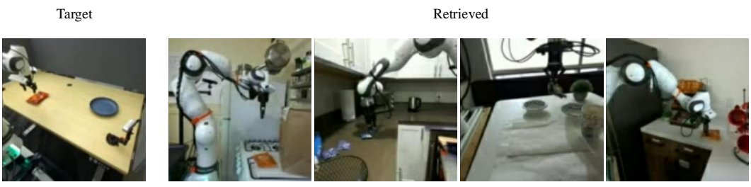
Figure 10: Retrieved cotraining demos for the serve snack task with the object spatial location aligned. The camera poses and textures seen in the demos are not the same as our target task, but the location of the object (in front of the robot and level with its base) is similar.
