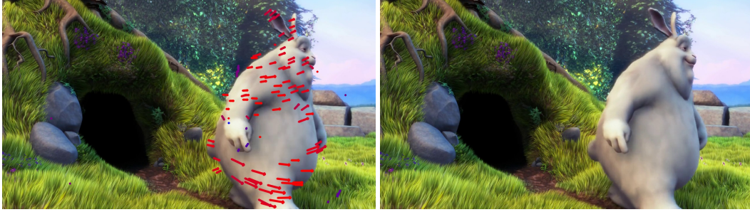
Figure 6: Illustration of motion vectors. The left figure is a snapshot from (Roosendaal, 2008) including a sub-sample of the motion vectors computed to the next frame (blue color corresponds to movement to the left and red corresponds to movement to the right), which is included to the right. Observe that while the most of vectors follow the movement, there is noise in the directions (either in magnitude or the direction of the moment) as evidenced by the small vector on a rock and a grass leaf in the left half of the image.
