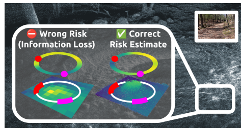
Figure 1. Dense point cloud captures geometric detail of the environment (Top right), while discretizing it into elevation map results in information loss. The underlying terrain is clearly distinguishable from noise (leaves, sensor noise) in the point cloud, but doing so is hard in an elevation map, leading to wrong risk estimation (Viridis Circle where Green denotes low risk).
