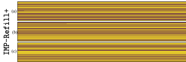
Figure A10: Sparse mask visualizations of the extreme winning tickets from IMP-Refill+ (channel-wise structural), and on (VGG-16,C10). The darker color indicates the remaining unpruned elements. (a,b,c) are the last three conv. layers.
