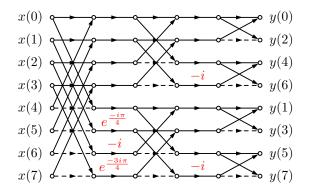
Figure 2: The 8-point fast Fourier transform signal flow graph. x and y represent the signal in the physical and Fourier domain, respectively. Dashed lines represent a multiplication by -1, red elements denote a multiplication by that factor, and converging arrows represent a sum.
