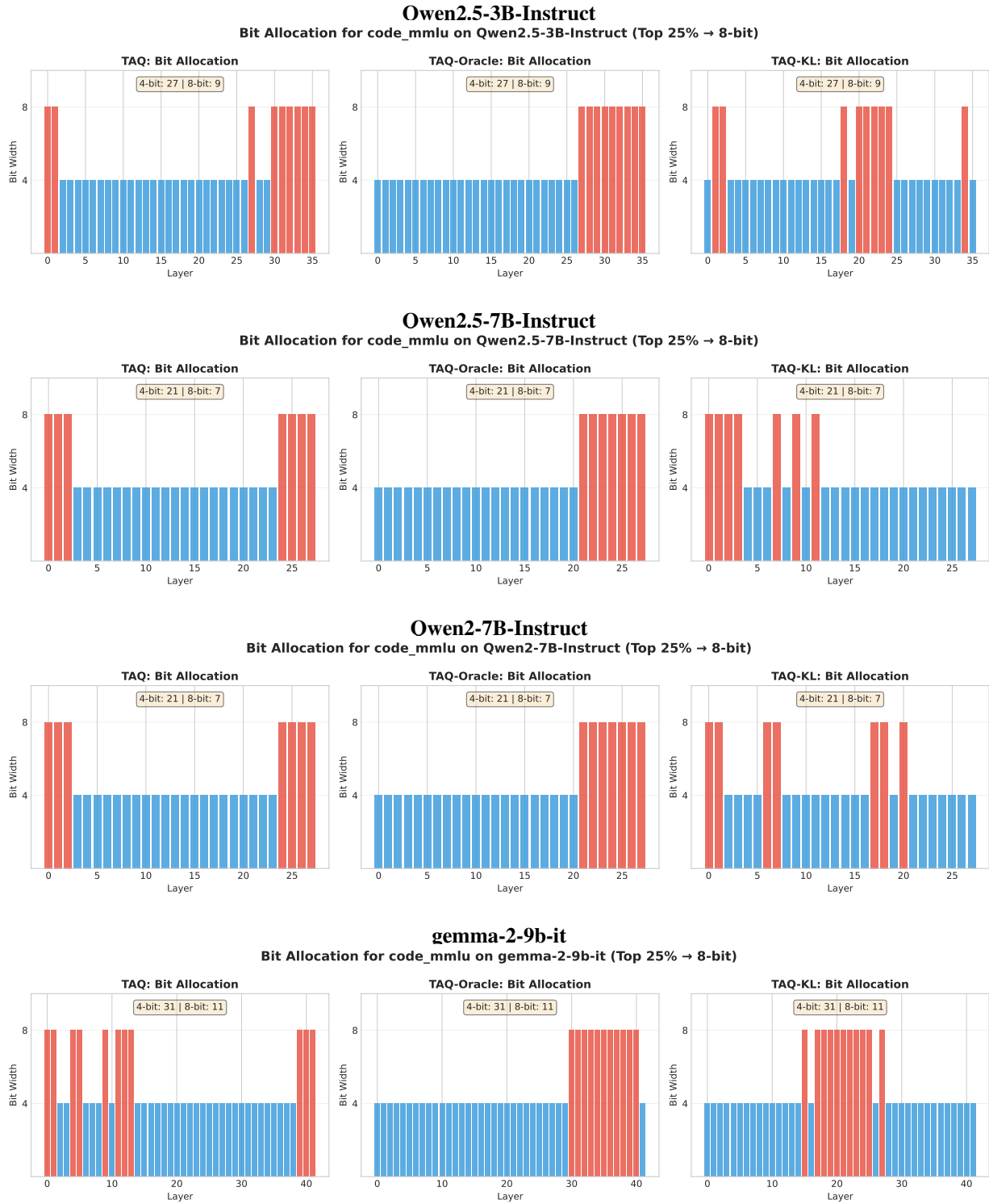
Figure 8. Layerwise mixed-precision allocations on CodeMMLU across models. Layers ranked in the top 25% by TAQ, TAQ-Oracle, or TAQ-KL are allocated 8-bit precision; remaining layers use 4-bit.
