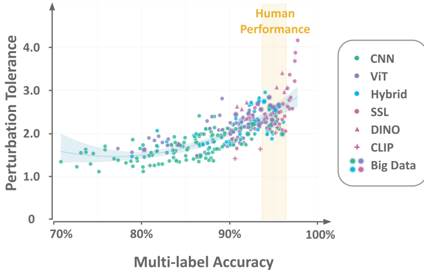
Figure 2: The Perturbation Tolerance of DNNs has significantly increased as they have improved on ImageNet. Each dot denotes a DNN’s performance on multi-label ImageNet (Shankar et al., 2020) vs. its average \ell_2 robustness radius to \ell_2 minimum-norm attacks, which we call Perturbation Tolerance . Error bars denote standard error, and the variance is so small for some models that it is invisible. The yellow region represents human performance, with mean=95.14% and std=2.02%.
