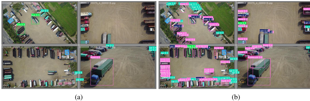
Figure 2: Output of the pre-trained model (a) and the fine-tuned model (b) for identifying types of vehicles.
