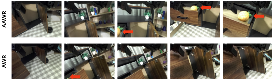
Figure 5: Example rollouts of AAWR vs AWR in the cabinet shelf task. AAWR explores the top left of the cabinet and locates the target object while AWR fails to adequately explore the full scene.
