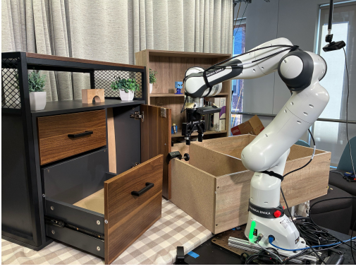
Figure 8: Robot hardware configuration: Franka Panda arm with wrist & side view camera.
