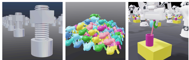
Fig. 2. Simulation scenes used for benchmarking. Left: an M20 nut-and-bolt assembly [5] Center: a pile of 91 colliding nonconvex bunny meshes, Right: a Franka Panda robot grasping a pen and placing it into a cup. For the nut-and-bolt and Panda scenes, we use MjWarp [12] and simulate 128 and 512 independent instances in parallel, respectively; for the Bunny Pile, we use Newton's XPBD.
