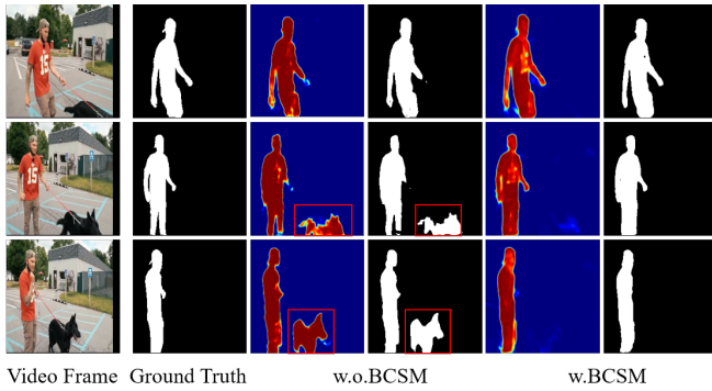
Figure 5: Comparison of features between the two versions. As depicted, feature maps without BCSM show substantial responses to interfering objects such as the dog, while BCSM effectively suppresses these responses.
