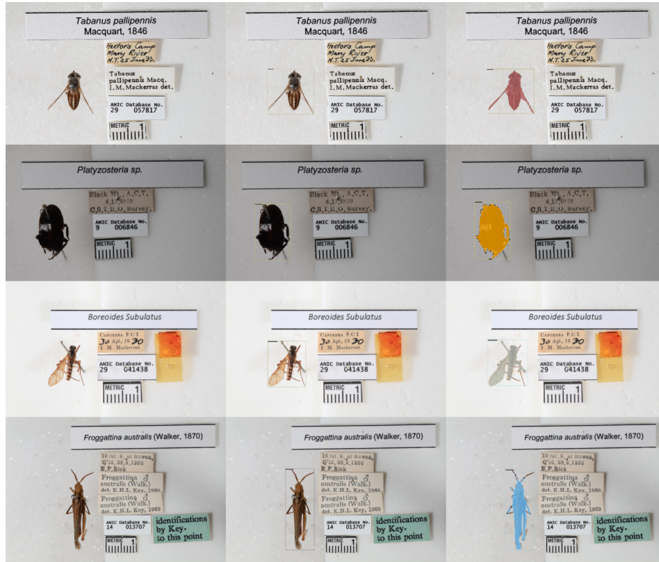
Figure 4: Qualitative detection and segmentation results. From left to right: original image, bounding box predicted by DINO, and instance mask predicted by Mask R-CNN.
