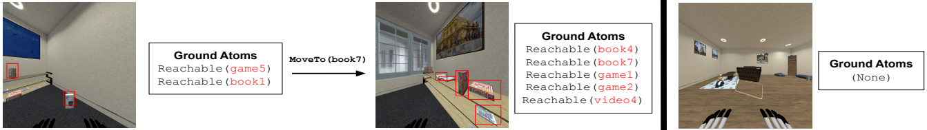
Fig. 1. Example demonstration transition and evaluation task from BEHAVIOR-100. (Left) Visualization and high-level states for an example transition where the agent moves from being in range of picking a number of objects. (Right) Visualization of an evaluation task where the agent starts out not in range of picking any objects.
