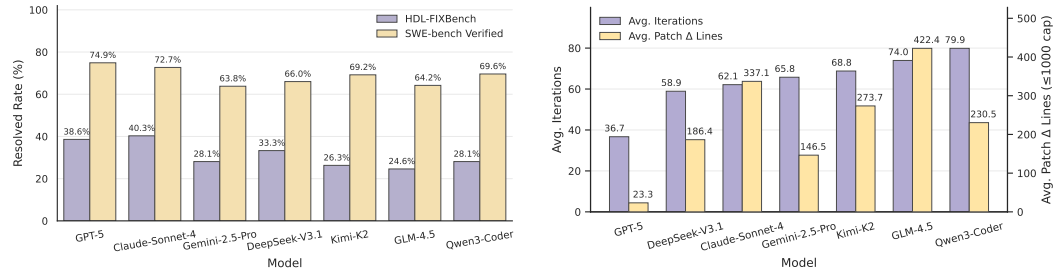
(a) Resolved rates on HDL-FixBench versus SWE-bench Verified across models. (b) Average number of agent iterations and lines changed (patch size capped at 1,000 lines).
