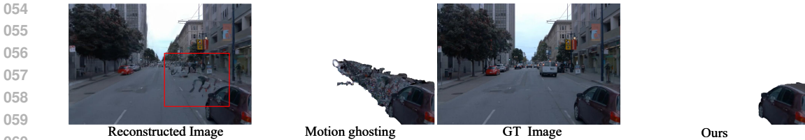
Figure 1: Qualitative visualization of dynamic ghosting in instance-level rendering. When modeling dynamic objects, the model tends to generate ghosting artifacts of the object at different positions. Our method effectively addresses this issue at the instance level. GT denotes the ground truth.
