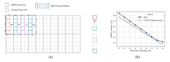
Figure 10: (a) Illustration of how we implement our GeMV Kernel to exploit activation sparsity. (b) Performance of our GeMV implementation in comparison to the perfect scaling.
