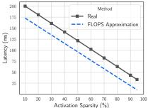
(a) sparse vector, dense matrix multiplication: by skipping rows, we reduce both the weight transfer (i.e., loading these rows for computation) and computation (i.e., the result will be zero).
