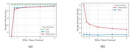
Figure 8: The effect of shifted ReLU on Llama model. (a) The performance is almost the same as the original ReLU. (b) Shifted ReLU (i.e., ReLU(x - 1)) is much sparser than the original ReLU.
