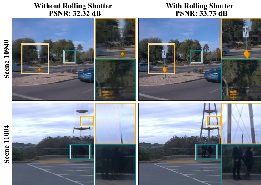
Figure 10: Rolling Shutter. Images captured from fast-moving vehicles such as those in the Waymo Open Dataset (Sun et al., 2020) exhibit rolling shutter effects that, when unaccounted for, degrade reconstruction quality ( left ). Our rendering formulation incorporates sensor movement into the projection function and evaluates the particle response function in 3D using the exact timestamp of each ray, allowing us to model time-dependent effects at high granularity ( right ).
