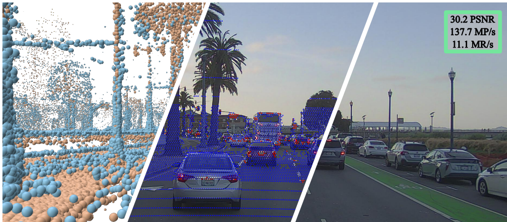
Figure 1: SimULi . We design a factorized 3D Gaussian representation that encodes camera and LiDAR information into separate sets of 3D Gaussians joined via nearest-neighbor anchoring loss ( left ). To efficiently render LiDAR scans ( middle ), we extend 3DGUT (Wu et al., 2025b) with an automated tiling strategy and ray-based culling. When compared to existing methods, we render 1.5-20 \times faster and match or exceed LiDAR and camera quality ( right ) across a wide range of metrics.
