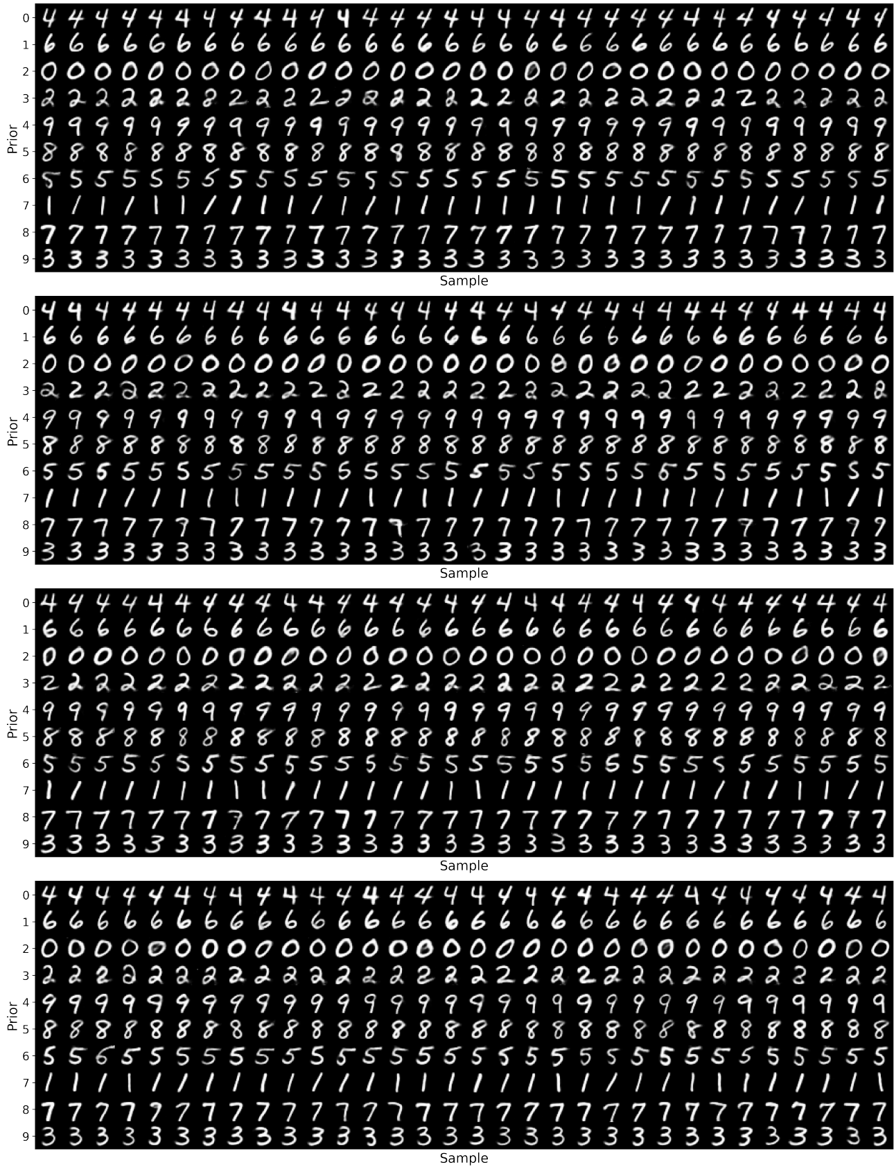
Figure 13. Various samples from each of the generative priors. Each prior learns to represent one of the digits. Further, we see a lot of variation between the different samples, suggesting that the clusters of the DRPM-VC manage to capture some of the diversity present in the dataset.
