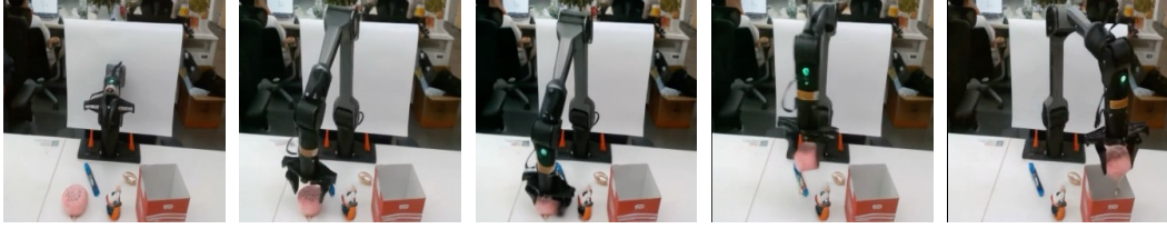
Figure 5: Real-world rendering results of world simulator. We show a video sequence generated by our world simulator in real-world scene.
