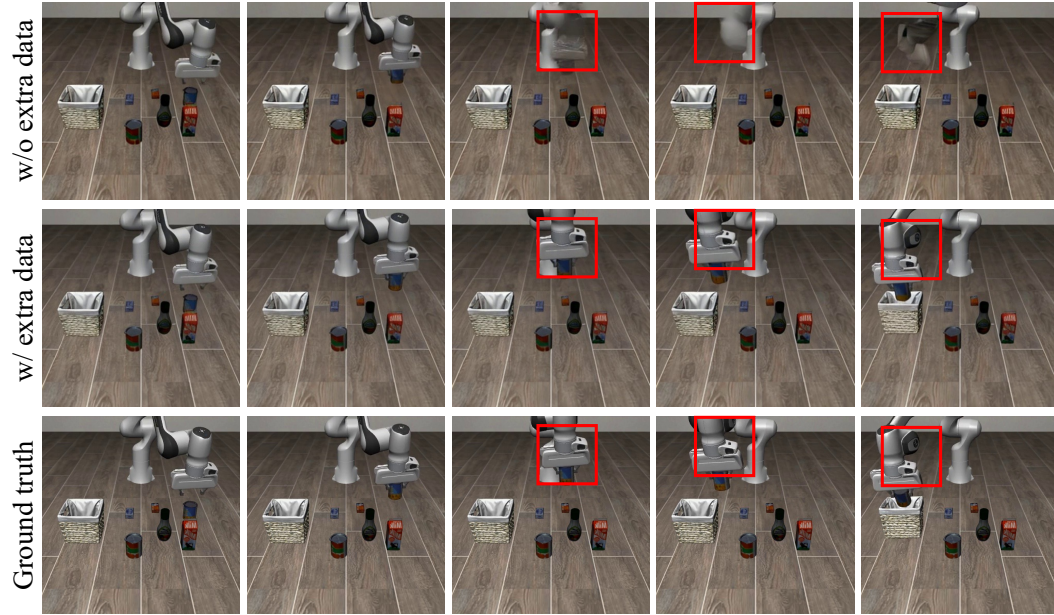
Figure 4: Rendering comparison of world simulator trained with and without extra data.
