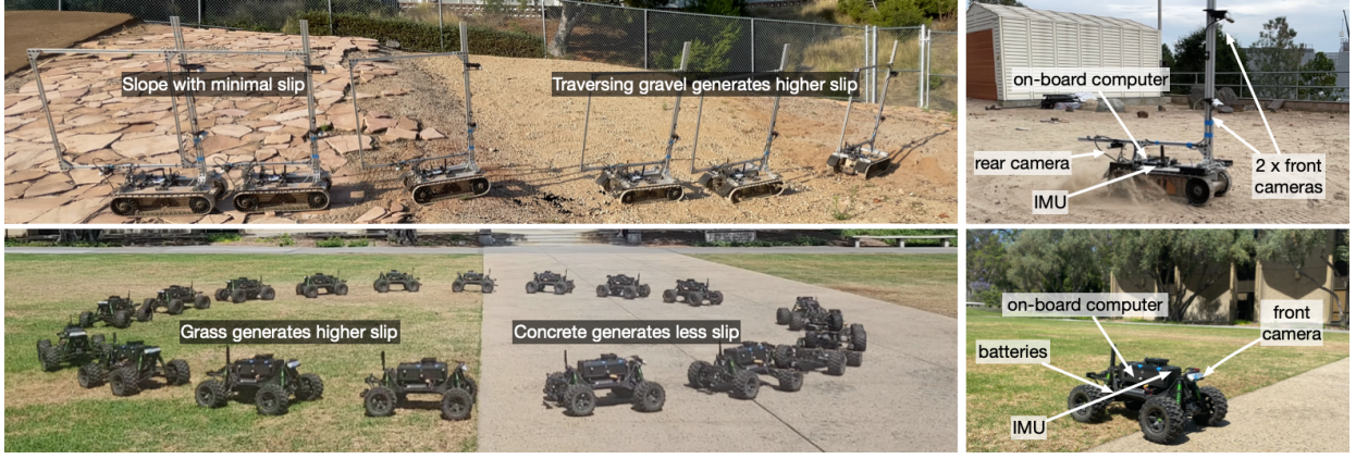
Fig. 12: a) The GVR-Bot traversing two slopes with different textures and terrain-induced dynamic behaviors at the JPL Mars Yard. b) The GVR-Bot with the sensing and compute units highlighted. Note that the forward facing camera is used for state estimation, while the top camera is used for taking terrain images for MAGIC VFM . The rear camera is not used in this work. c) The Traxxas robot traversing two different terrains that induce different dynamic behaviors. d) The Traxxas robot with its main sensing and compute units highlighted.
