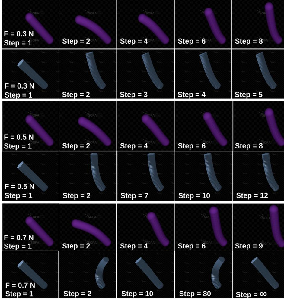
Figure 22: A comparison between the proposed solver embedded in SOFA shown in purple and SOFA’s native Cosserat rod plugin.
