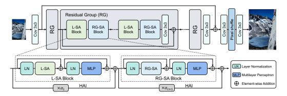
Figure 1: The architecture of the Recursive Generalization Transformer (RGT). The local selfattention (L-SA) blocks, and recursive-generalization self-attention (RG-SA) blocks are alternately arranged.  $\alpha_l$  is a learnable adaptor in the hybrid adaptive integration (HAI) of the  $l^{th}$  block.
