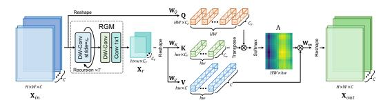
Figure 2: The illustration of the recursive-generalization self-attention (RG-SA). The RG-SA first generates the representative feature maps with constant size  $(h \times w)$ , through the recursive generalization module (RGM). Then, the cross-attention between input features and representative maps is performed to capture global information.  $\otimes$  denotes matrix multiplication.
