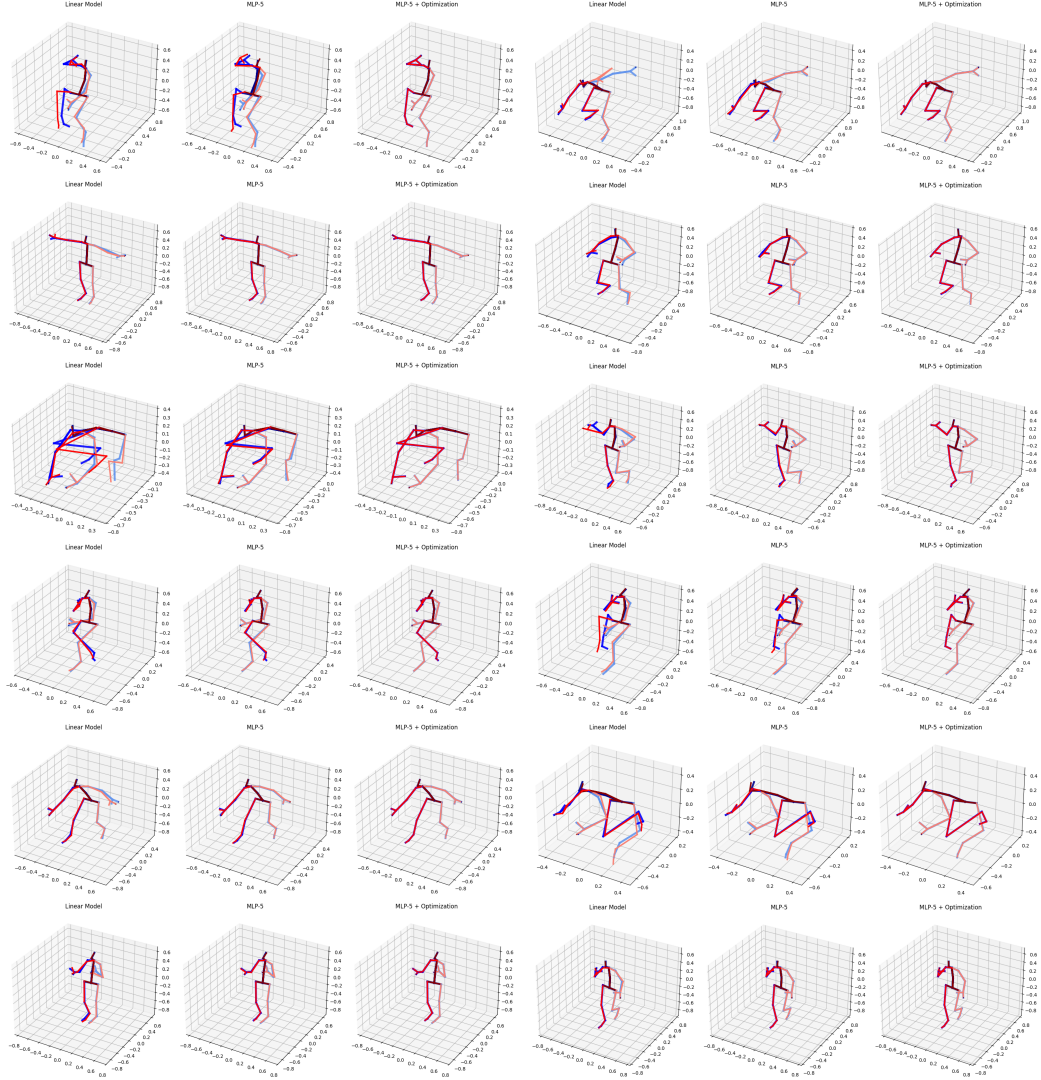
Figure 12: Results of the learned inverse kinematics on the unseen Human3.6M test set are presented. The blue skeletons represent the ground truth 3D projections, while the red skeletons correspond to the predictions obtained by applying forward kinematics to the articulated pose parameters. We compare the outputs of a linear model, our 5-layer MLP, and gradient descent-based post-optimization. The first row highlights two failure cases with the highest errors across the test set. Notably, even the linear model produces reasonable predictions in many challenging examples. The direct output of the MLP closely matches the ground truth, and the post-optimization step further refines the alignment, achieving the most accurate results.
