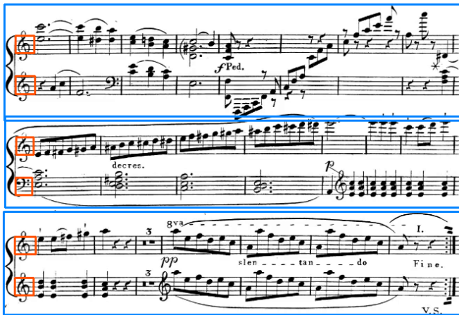
Fig. 6. Illustration of the music system detection pipeline using the fine-tuned YOLOv8 models. Detected systems are notated with blue boxes, and staff lines with red boxes. Note that the red boxes detect the staff height near clefs, not the clefs themselves.
