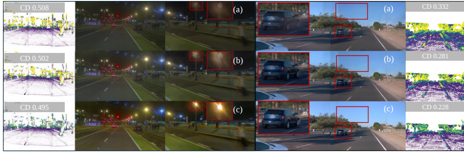
Figure 4: Our proposed framework (c) outperforms appearance codes (a) and single bilateral grids (b) by simultaneously addressing optimization challenges and enhancing geometric modeling. This delivers significant geometric accuracy improvements (lower Chamfer Distance (CD) via multi-scale bilateral grid, reducing error and improving reconstruction) and reduced photometric inconsistency (fewer floaters) in dynamic, decoupled driving scenes. Yellow indicates a high lidar error, while Purple indicates a low lidar error.
