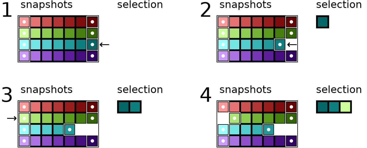
Figure 1: Bidirectional snapshot selection: The candidate pool is marked with light circles. The arrow marks the selected snapshot yielding the highest decrease in cross-validated loss. Its neighbour replaces it in the pool.
