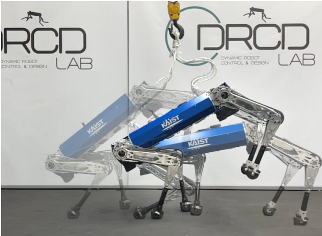
Figure 1. Experimental demonstration of front-leg rearing motion with the HOUND quadruped robot using the proposed framework. Only a desired body pitch angle was set, without any predefined contact modes.
