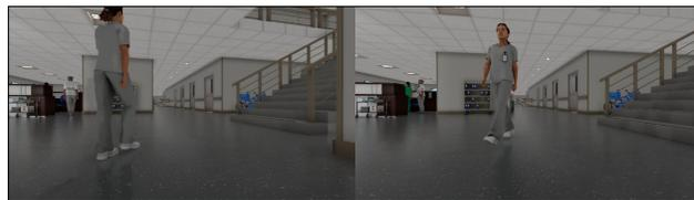
Figure 6. **Challenging case on SLAM.** This figure represents the failure case that occurred during evaluating SLAM algorithms on our dataset. In this case, invalid feature matching occurred due to the moving and dynamic object at different times.
