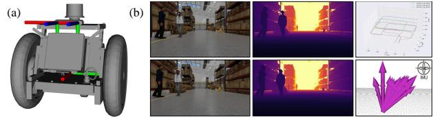
Figure 2. **Robot configuration and sensor data example.** (a) The NVIDIA Carter, our robot platform. (b) Examples of acquired sensor data (stereo RGB, stereo depth, GT poses and IMU).
