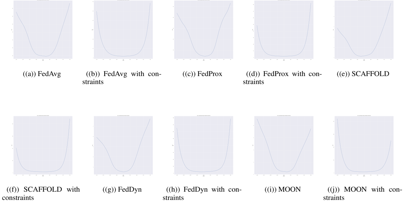
Figure 10. This figure presents the experimental results of the loss landscape for the ResNet-18 model in a cross-device setting of ???. Noise was introduced to the weight \|W\| in the form of a random vector \epsilon , scaled such that the ratio \|\epsilon\|/\|W\| ranged from 0 to 1. The results demonstrate that applying constraints leads to a more convex loss landscape, indicating an enhanced generalization capability under these conditions.
