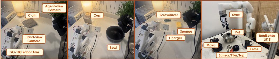
Figure 11: Real-world experimental setups. We conduct experiments on both SO100 and xArm platform. For each robot, we design a suite of 10 tabletop tasks involving diverse objects.
